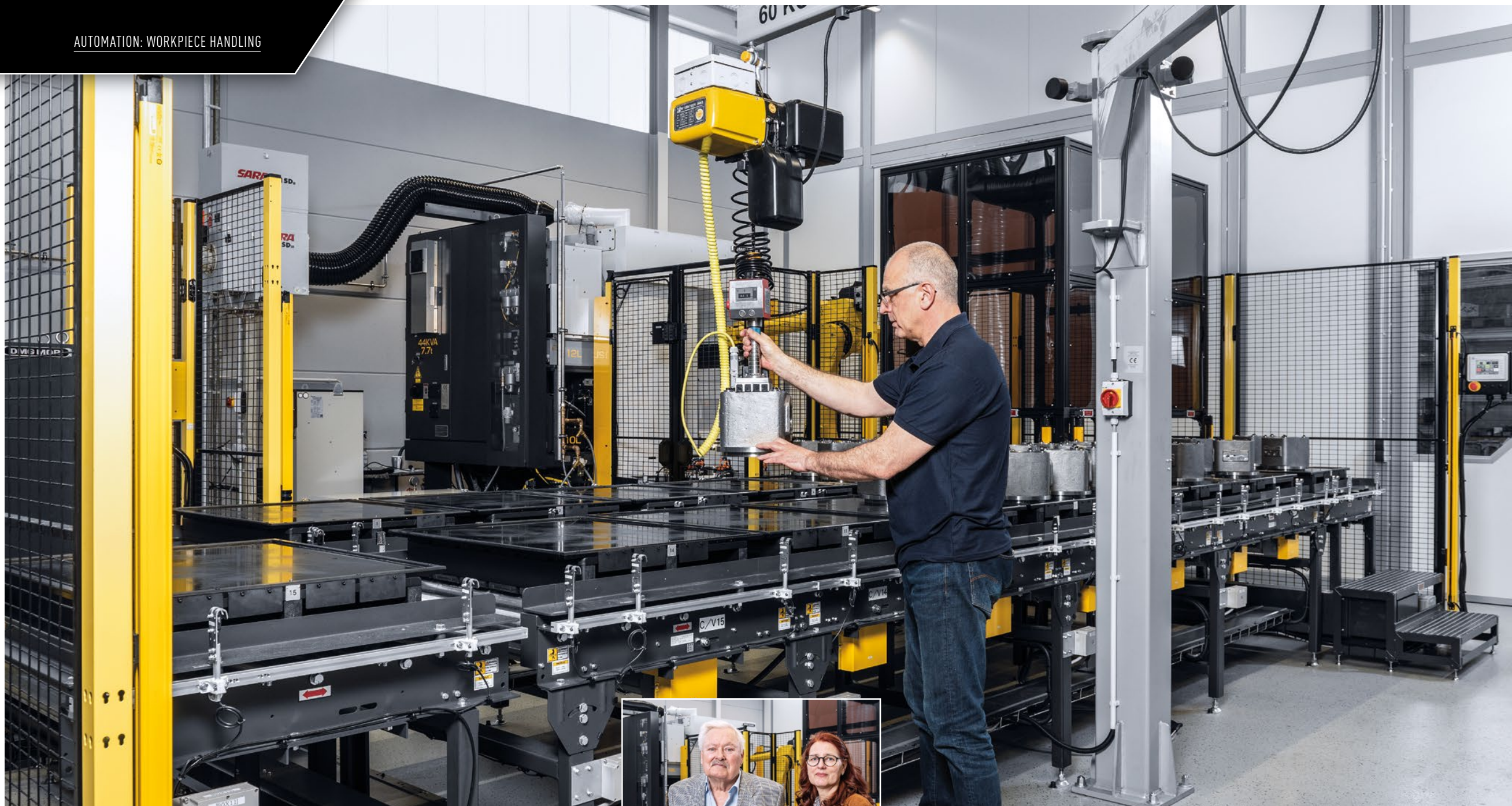
A camera captures the exact position of the components on platforms. The robot grips the workpieces with precision based on the images.
