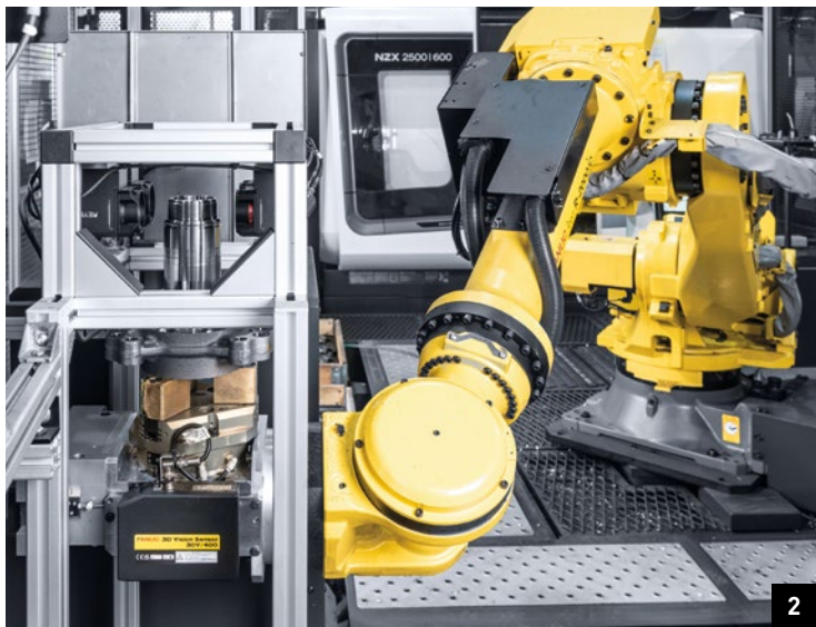
1. The modular design of the MATRIS enabled the integration of a blow-off station and a station for optical measurement of the components. 2. The optical measurement station within the automated process checks and documents the bearing seats, the thread core and the flank diameter of the stub axles.
