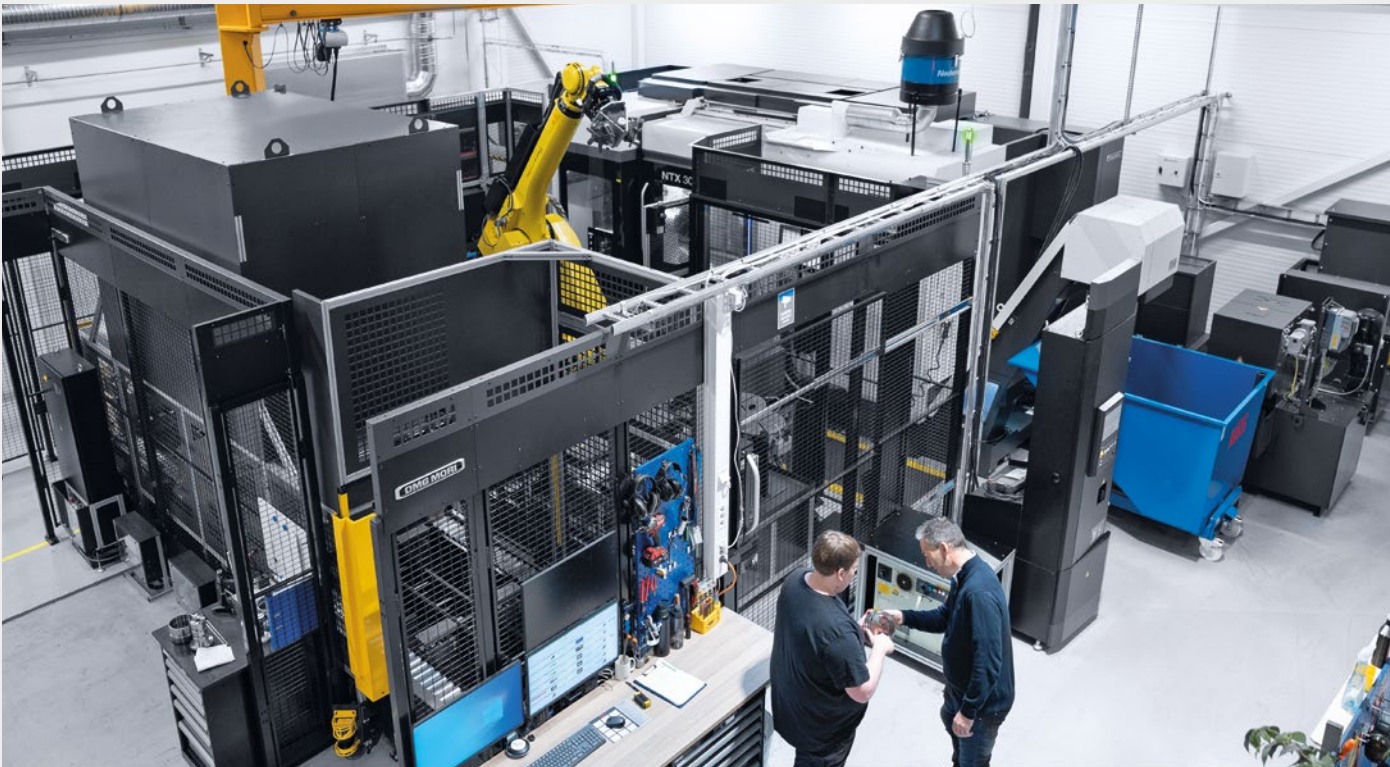
Thanks to the MATRIS workpiece handling system, the NTX 3000 now operates over two unattended shifts. And it does so with a high degree of flexibility for producing batch sizes of less than 15 parts.
