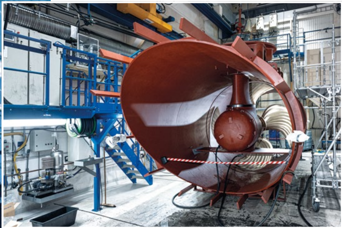
Among other things, Brunnvoll manufactures low-noise transverse thrusters that reduce noise by up to 15 dB.
