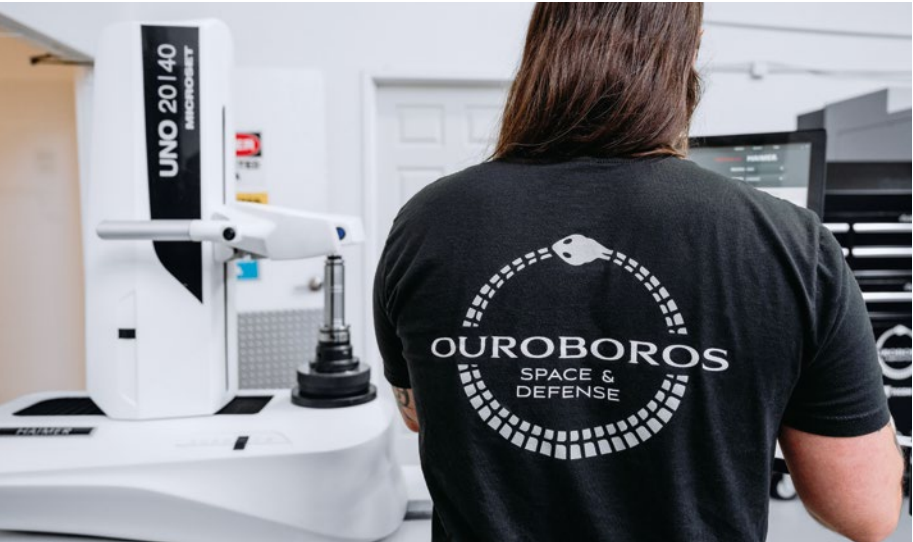
To achieve high precision tool offsets, Ouroboros used a tool presetter by DMPQ (DMG MORI Qualified Products) partner HAIMER.
