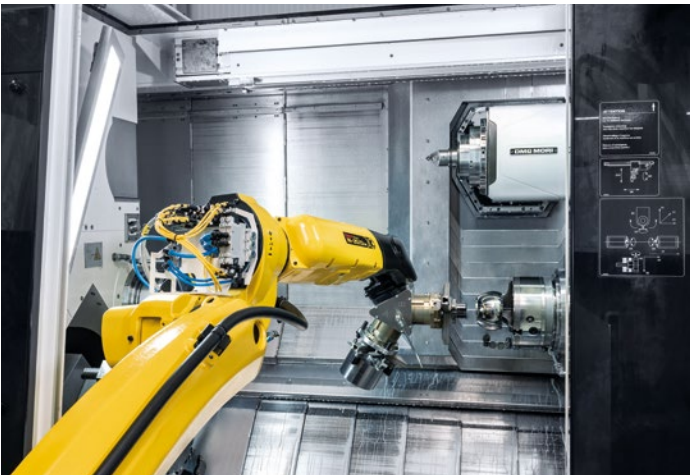
1. Machine transfers from main to sub 2. Robo2Go unload sub & loads main
