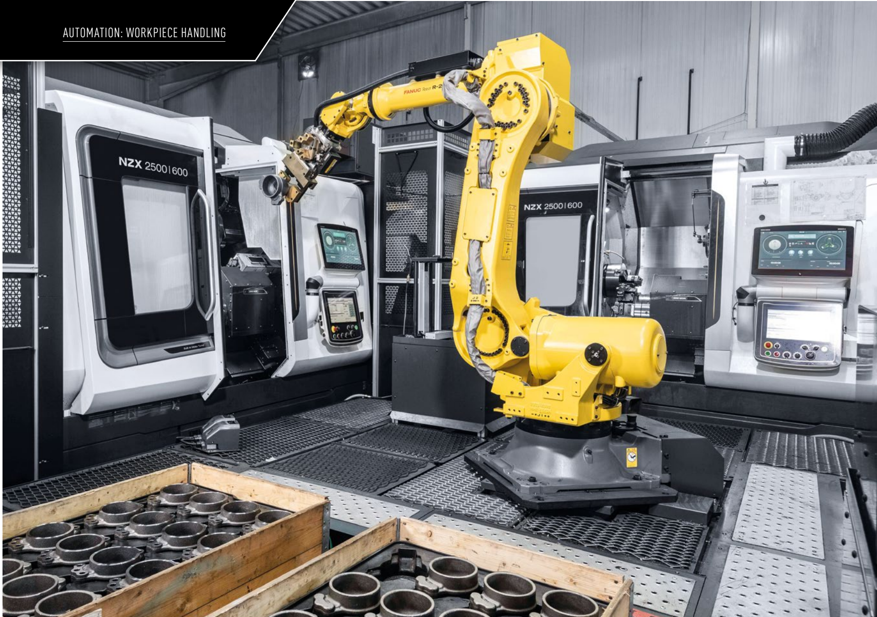
The robot with vision system loads and unloads the two NZX 2500s respectively with the left and right hand variants of the stub axles.
