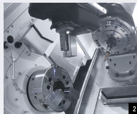
Can exchange chuck jaws inside the machine
