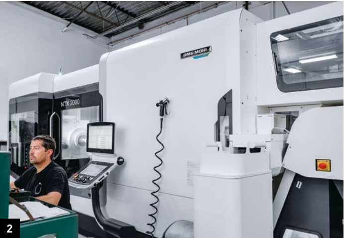
1. Part of the Ouroboros team in front of the NTX 2000 2. The NTX 2000 enable 6-sided turn & mill complete machining of workpieces up to \varnothing 670 \times 1,538 mm 3. For smaller components up to up to \varnothing 630 \times 600 mm and 300 kg, Ouroboros uses a DMU 50 3 rd Generation
