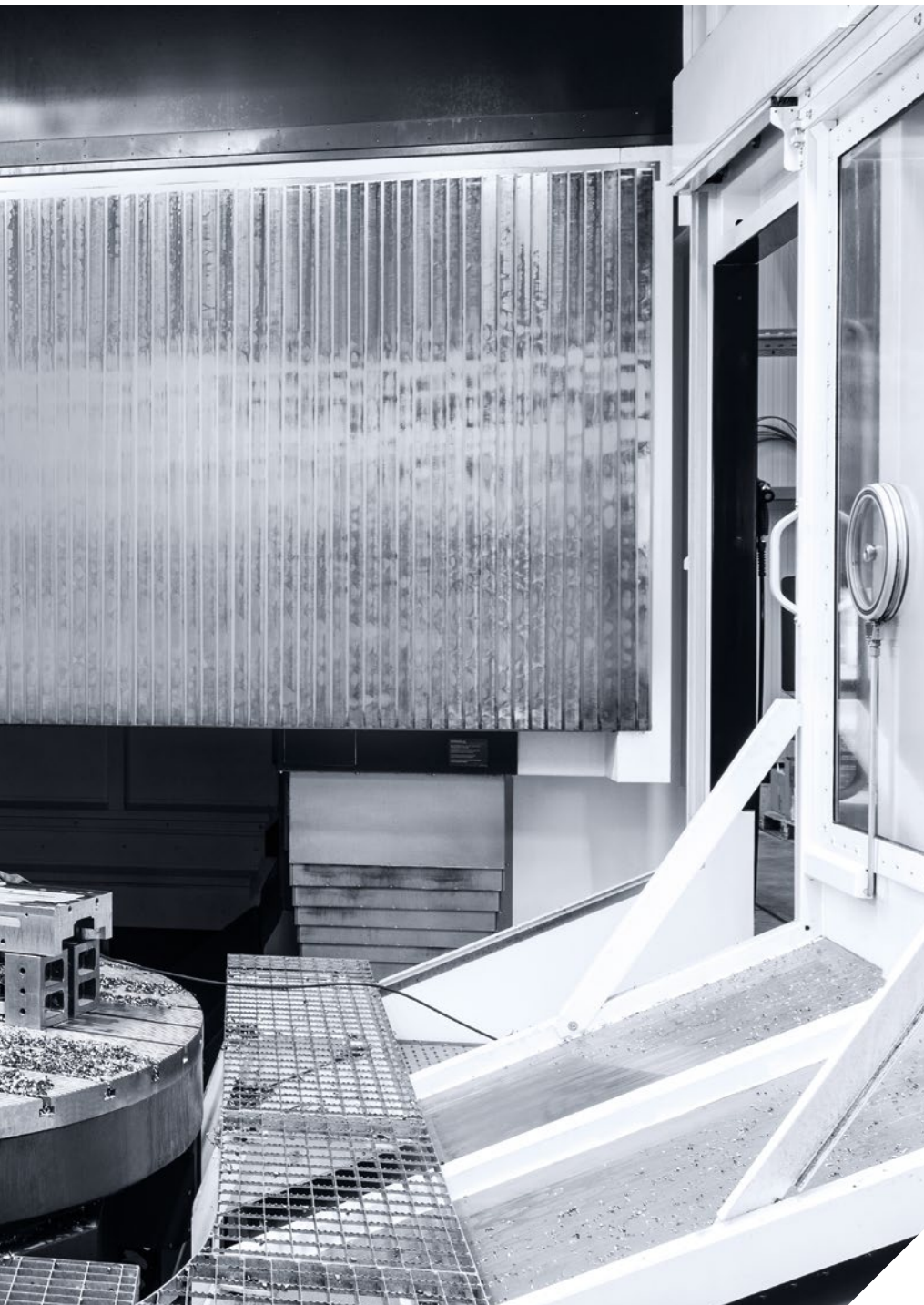
The work area of the DMU 340 P measures 3,400 × 3,400 × 1,600 mm. Maximum table load is 16 t.
