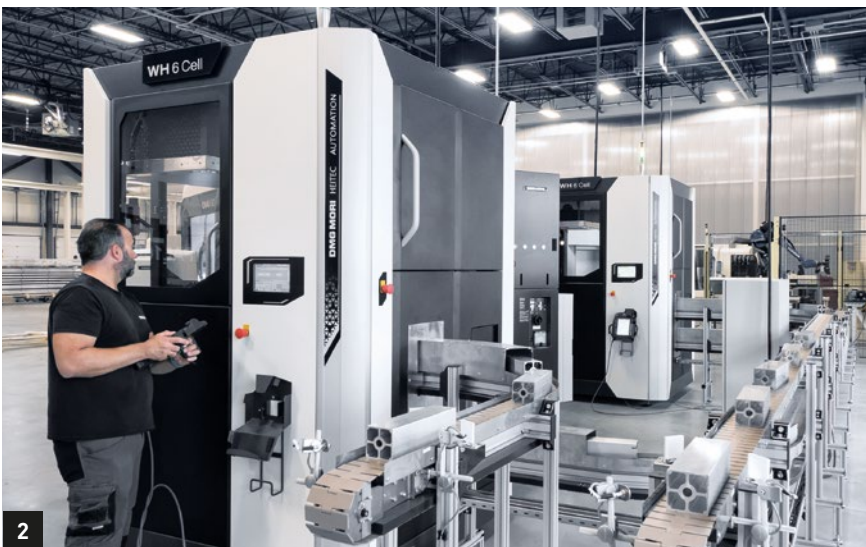
1. Automated manufacturing allows Attabotics to meet its high demand for base columns and other components, even at full capacity. 2. The automated loading and unloading of the DMU 50 3 rd Generation achieves high production capacity and more manufacturing flexibility.
