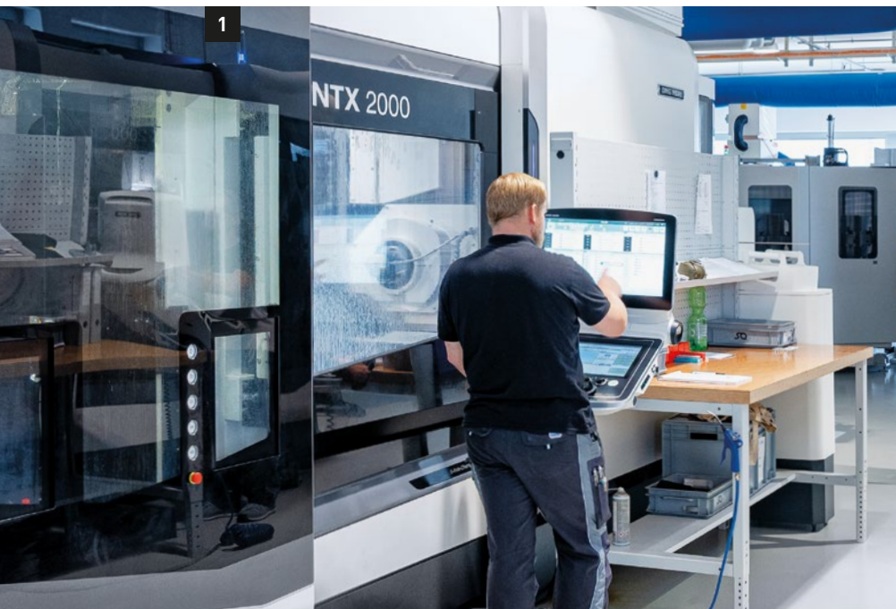
1. SQ Products has so drastically optimized production processes with its total of six NTX 2000 centers that throughput times for the sockets of a shoulder implant have been reduced from what often took several weeks to just one day. 2. SQ Products meets the highest accuracy requirements during the production of medical implants.
