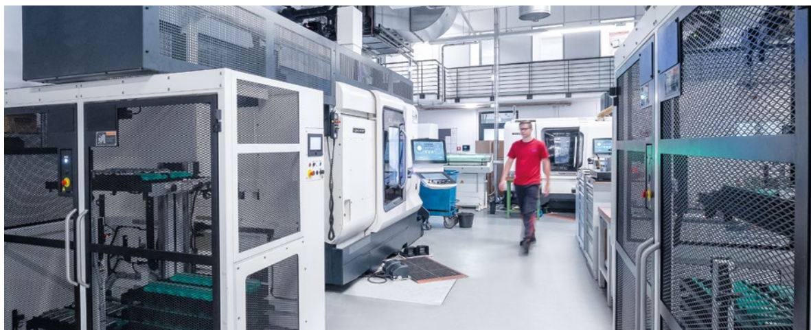
The two GX 10 T gantry loaders serving the NZX 2000 and NLX 2500 and the bar loader of the NLX 2000 enable efficient multiple machine operation.
