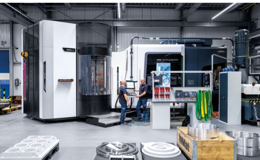
Equipped with grinding capability, the DMC 125 FD duoBLOCK achieves surface qualities down to 0.4 \mu\text{m} Ra and circularity of 5 \mu\text{m} .
