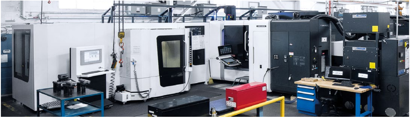
Included in Top Grade Molds' fleet of machines are four NHX 5000s, which operate automatically with two linear pallet pools.
