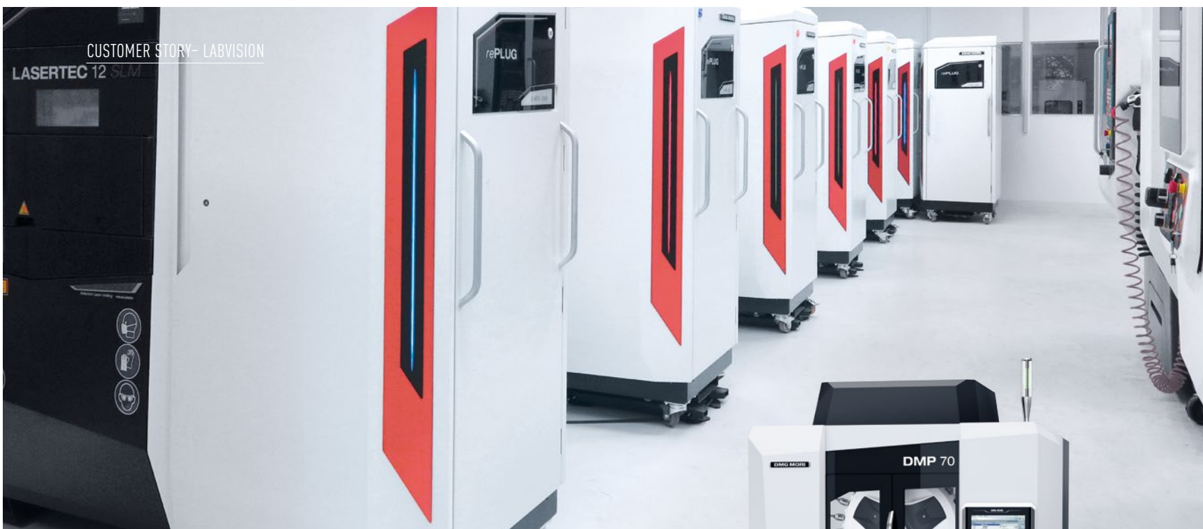
Additive manufacturing and high-precision milling: With six LASERTEC 12 SLM , two DMP 70 and one MILLTAP 700, LABVISION has established a hybrid process chain in dental technology.
