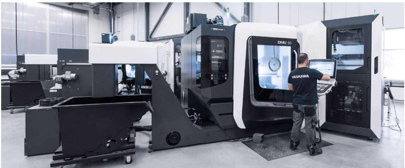
With automated production on the DMU 50 equipped with a WH 6 Cell, Attabotics meets the high demand for base columns and other components, even when at full production capacity.
