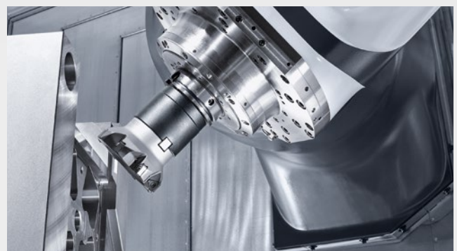
speedMASTER spindle with 20,000 rpm and 96 ft lbs | 47 hp (40 % DC).
