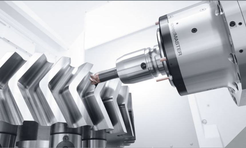
2.2 second chip-to-chip time, 0.5 sec. tool change time
