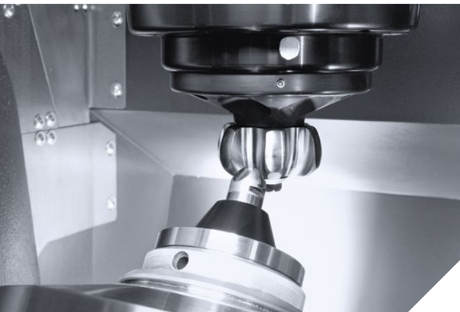
5-axis milling of an inner ball race on the CTV 250 DF.
