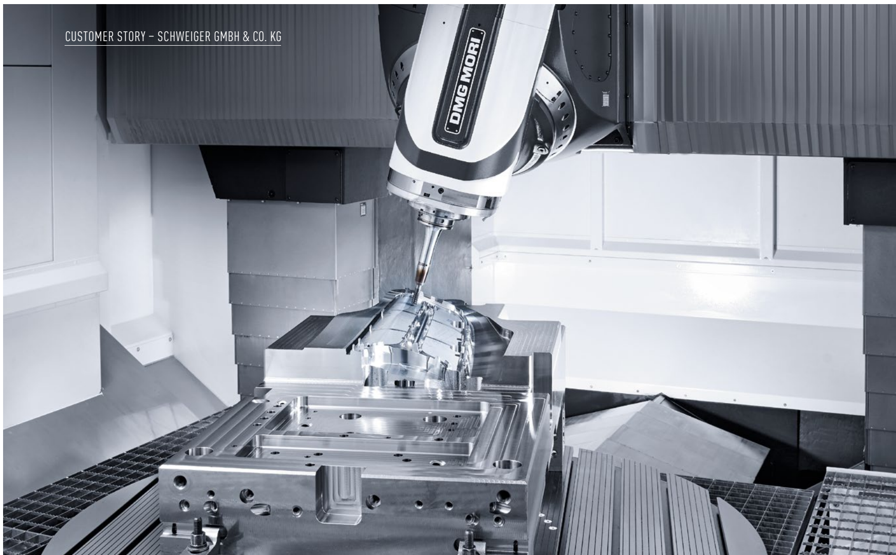
High-precision mold machining on a DMU 210 P.
