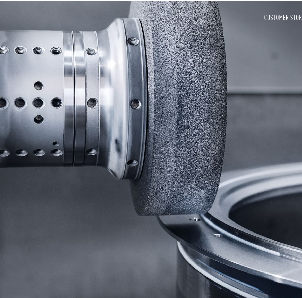
DMC 125 FD duoBLOCK including grinding package combines milling, turning and grinding in a single set-up.
