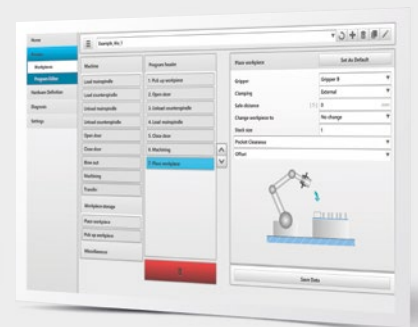
Programming screen for teaching robotic workpiece handling in <15 min
