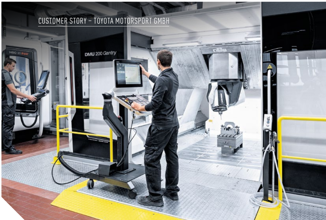
Installation of the DMU 200 Gantry in a pit to enable ground level loading and unloading of the delicate carbon fiber components with a forklift.
