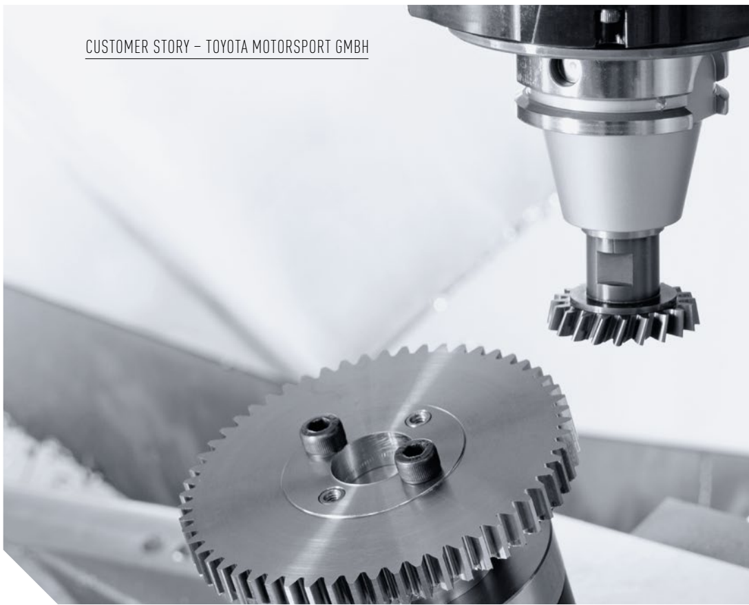
DMG MORI gearSKIVING – Machining of gears on a DMU 60 eVo to grinding quality.
