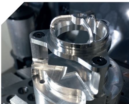
Example: High-precision valve seat for Andretti Autosport race cars, produced on the DMU 50 5-axis universal milling machine from DMG MORI.
