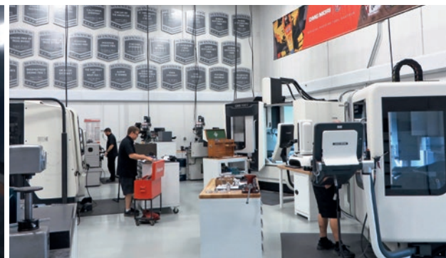
For the production of its race car parts, Andretti Autosport relies on turn-and-mill technology from DMG MORI, namely (from left to right) the NLX 2500 SY | 700, a CMX 1100 V and a DMU 50.
