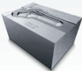
Forging die for hip nails Machine: DMC 650 V Material: 1.2343 Dimensions: 9.8 x 7.9 x 3.9 in.
