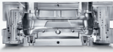
Mold insert for car bumpers Machine: DMU 600 Gantry linear Material: 21CrNiMo2 Dimensions: 98.4 x 39.4 x 55.1 in.
