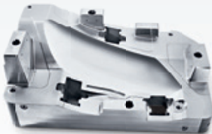
Injection mold for headlamps Machine: HSC 70 linear Material: 1.2312 Dimensions: 26.8 x 15.8 x 13.8 in. Ra < 0.15 μ
