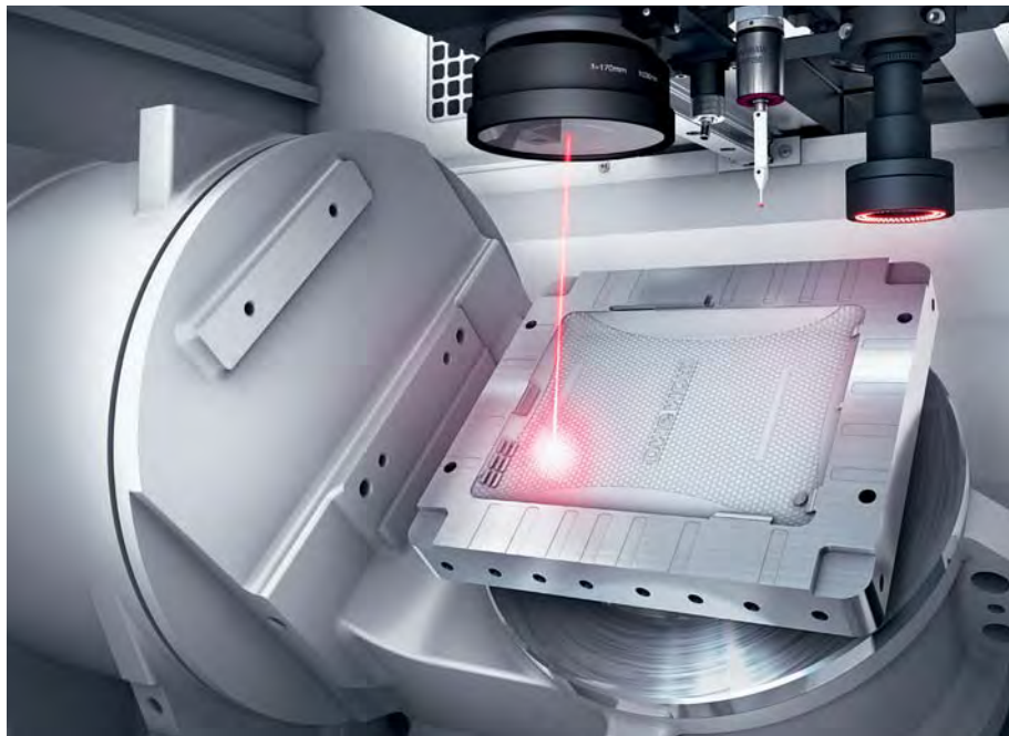
Work area of the LASERTEC 45 with an integrated swivel / rotary table (5-axis version), Laser head with a precision scanner, CCD camera and retractable measuring probe.
