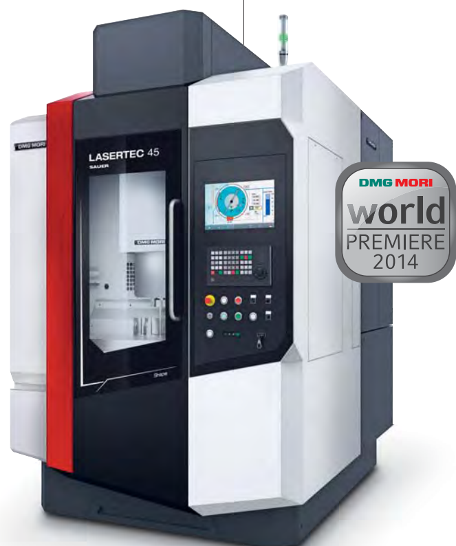
Laser ablation: intricate cavities for miniature molds
