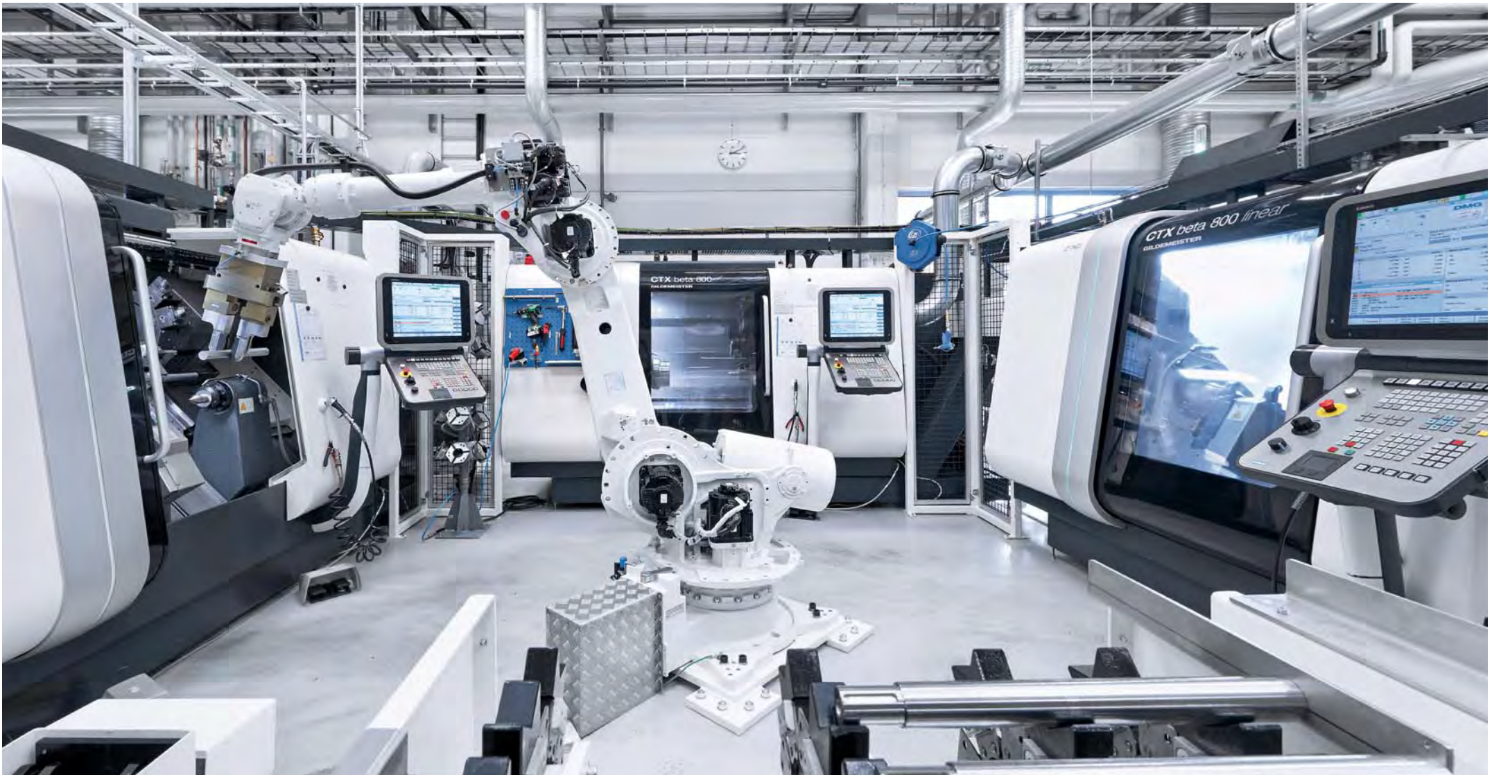
At the end of 2013, DMG MORI Systems installed a production cell at XYLEM consisting of 2 CTX beta 800 turning machines, 1 CTX beta 800 linear and a robot.
