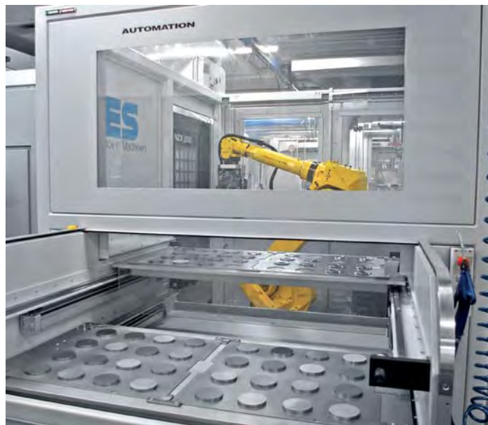
The integrated workpiece storage for parts up to 661.4 lbs. per drawer ensures safe and efficient delivery of blanks.
