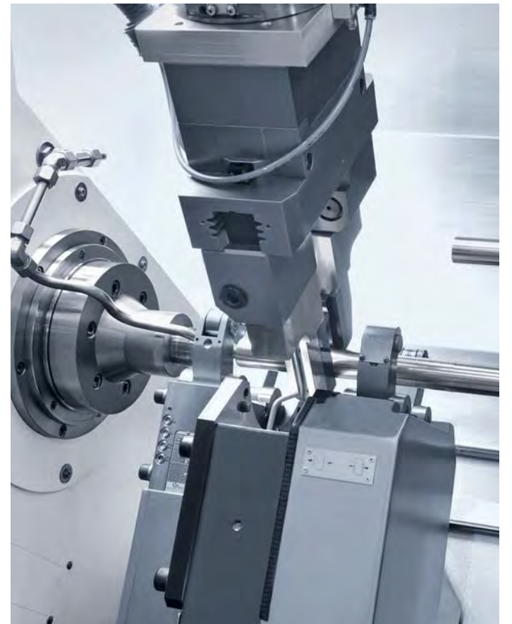
The steady rest of the CTX beta 800 linear stabilizes the workpiece during subsequent groove and drill hole operations.
