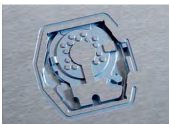
Laser ablation: intricate cavities for miniature molds
