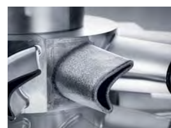
Laser deposition welding and milling of turbine blades
