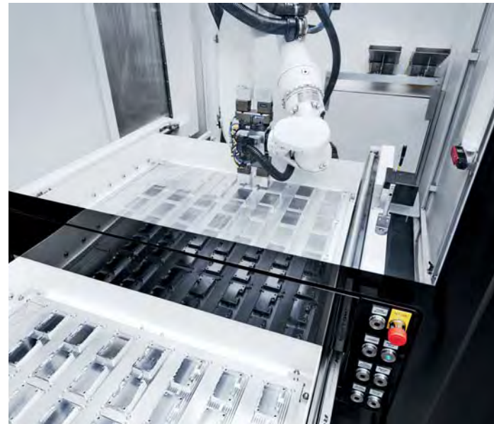
The workpiece storage with 2 drawers offers ample space for longer unmanned production phases.
