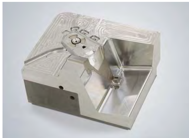
RC 50 Die-Var cavity insert showing high finish and detail attainable with HSC Technology.
