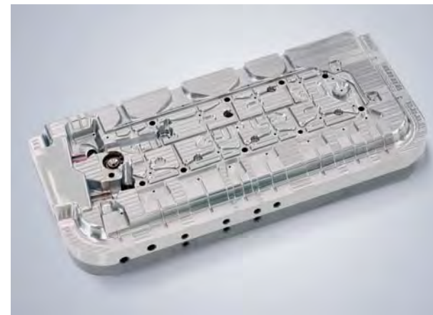
Complex die-cast cavity block machined to a level of finish requiring significantly less polishing time than in the past.
