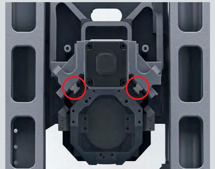
Greatest stability with two, angled guides positioned outside of the chip disposal area.
