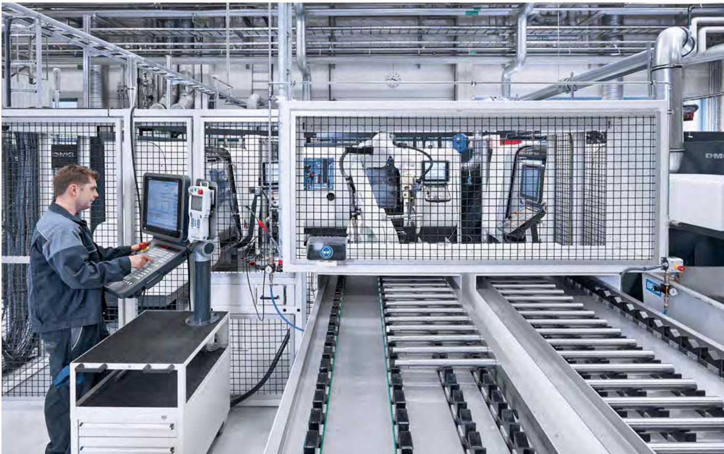
Two conveyor belts handle loading and unloading of the production cell. All other processes, including workpiece measuring, are carried out automatically, eliminating the need for final inspection.
