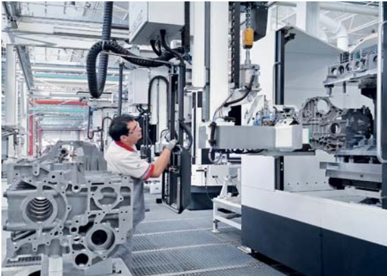
Workpieces are loaded at the setup point. In the foreground is a turning station.
