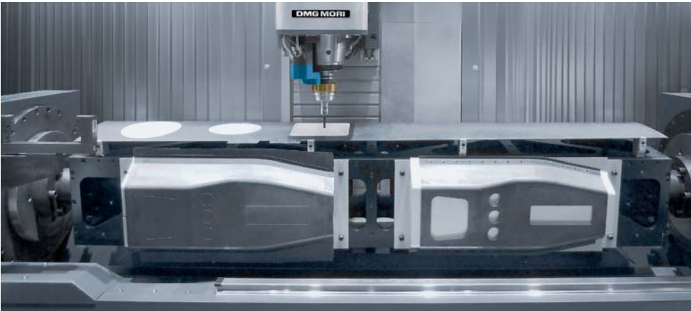
ULTRASONIC 260 with advanced technology and a custom clamping device: trimmings for rotor blade parts; splicings, drillings and pockets for a CFRP center console.
