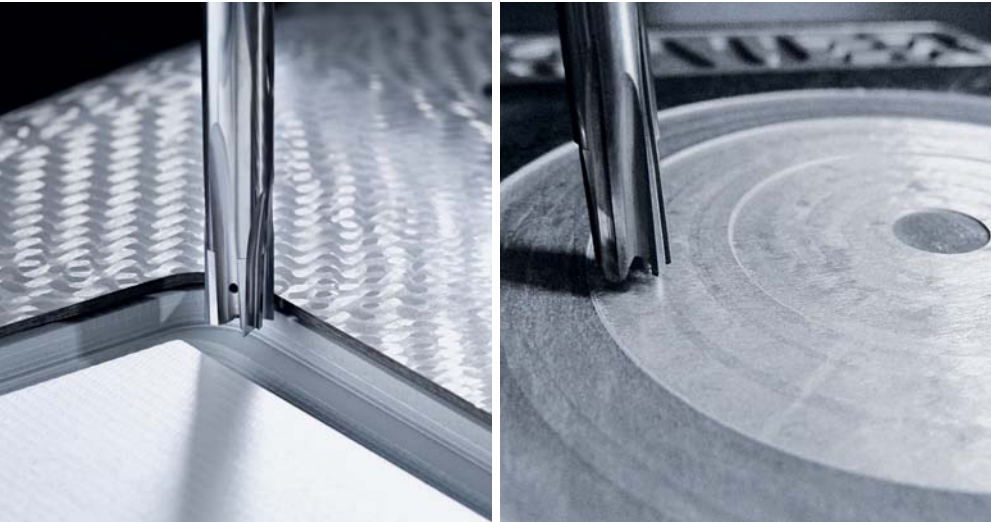
Carbon fiber splicing and trimming without edge chipping, fiber tearing or delamination.
