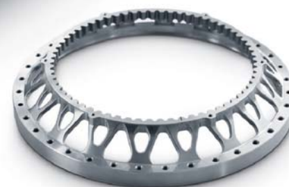
Brake disk hub Turning on a CTX beta 800 Milling on a DMU 80 eVo linear Material: Titanium Production time: approx. 7 hrs. (5-axis milling)
