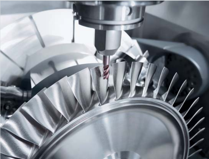
Impressive stability and dynamics of the monoBLOCK® Series are ideal for the production of blisk components.
