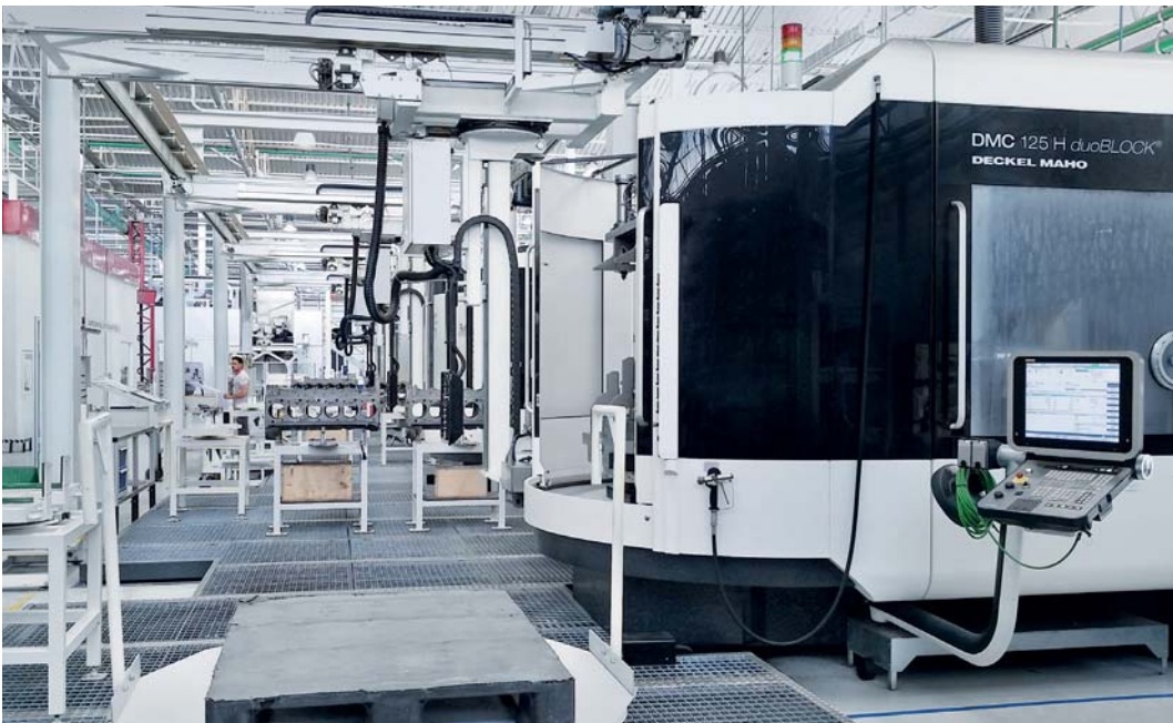
For FPT Industrial Argentina S.A., DMG MORI Systems developed a turnkey project with 13 DMC machining centers.
