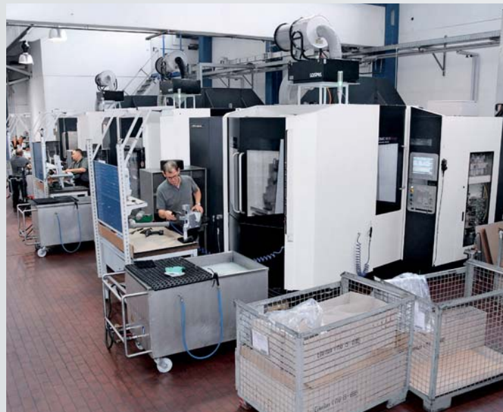
Three new DMC 60 H linear machines at ZBG produce challenging motorcycle parts quickly time with exceptional quality.
