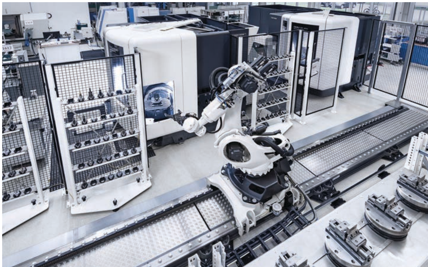
Flexible manufacturing cell with two DMU 60 eVo units, one DMU 70 eVo, one 7-axis CAD / CAM coupled robot and the master computer for controlling the machine, tool demand and job prioritization.
