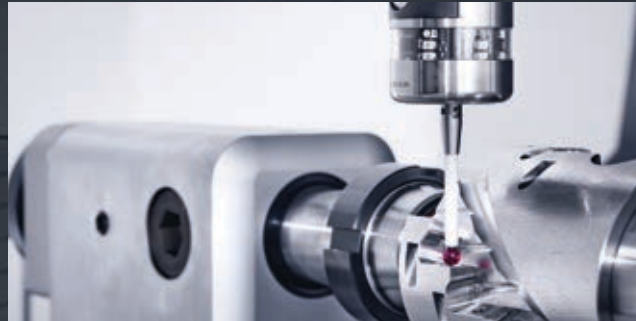
OPTION // NC-rotary table for efficient 4-sided machining
