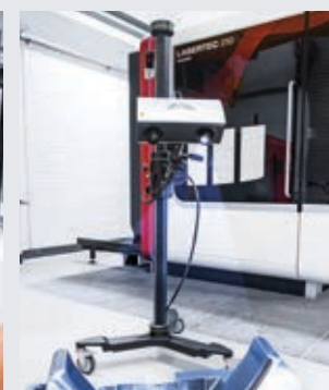
Measuring tool geometry using a 3D scanner.
