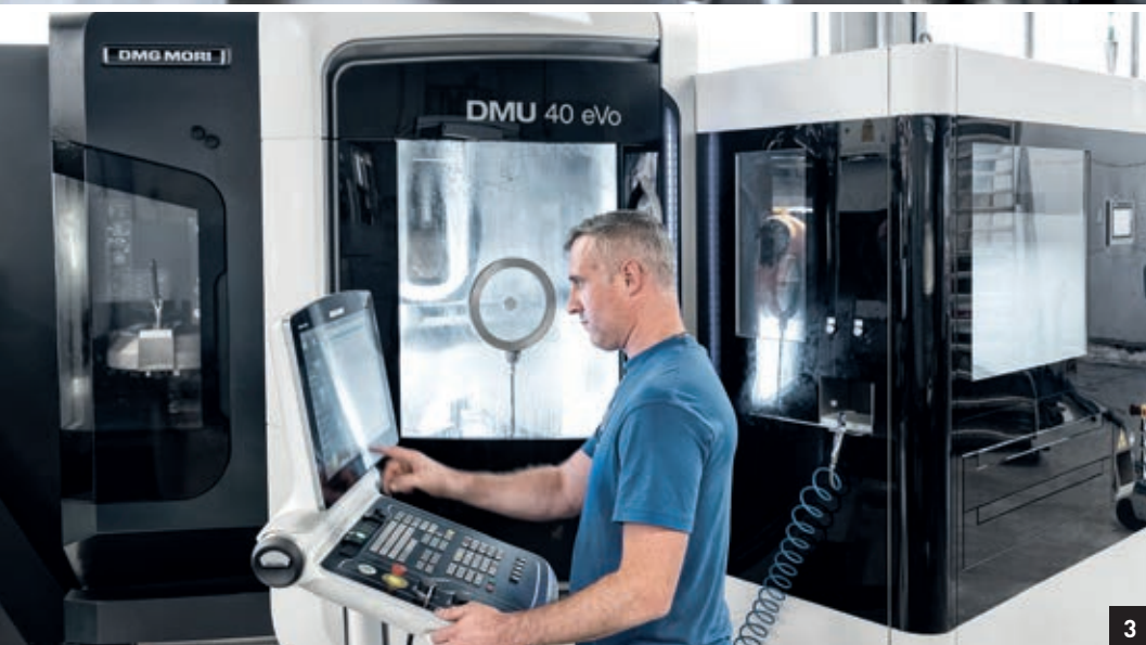
1. The DMG MORI production cell was developed as a dedicated turnkey project for vane machining 2. Accurate results to a tolerance of less than thousands of an inch in 3-shift operation 3. Perfect accessibility, also for manual operation
