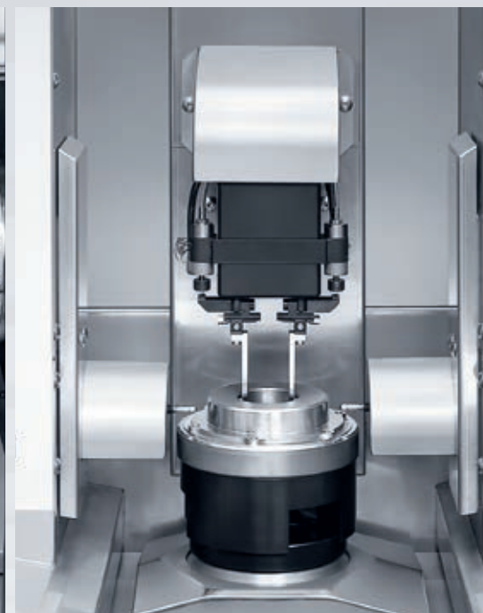
Inspection station for in-process measurement during production.
