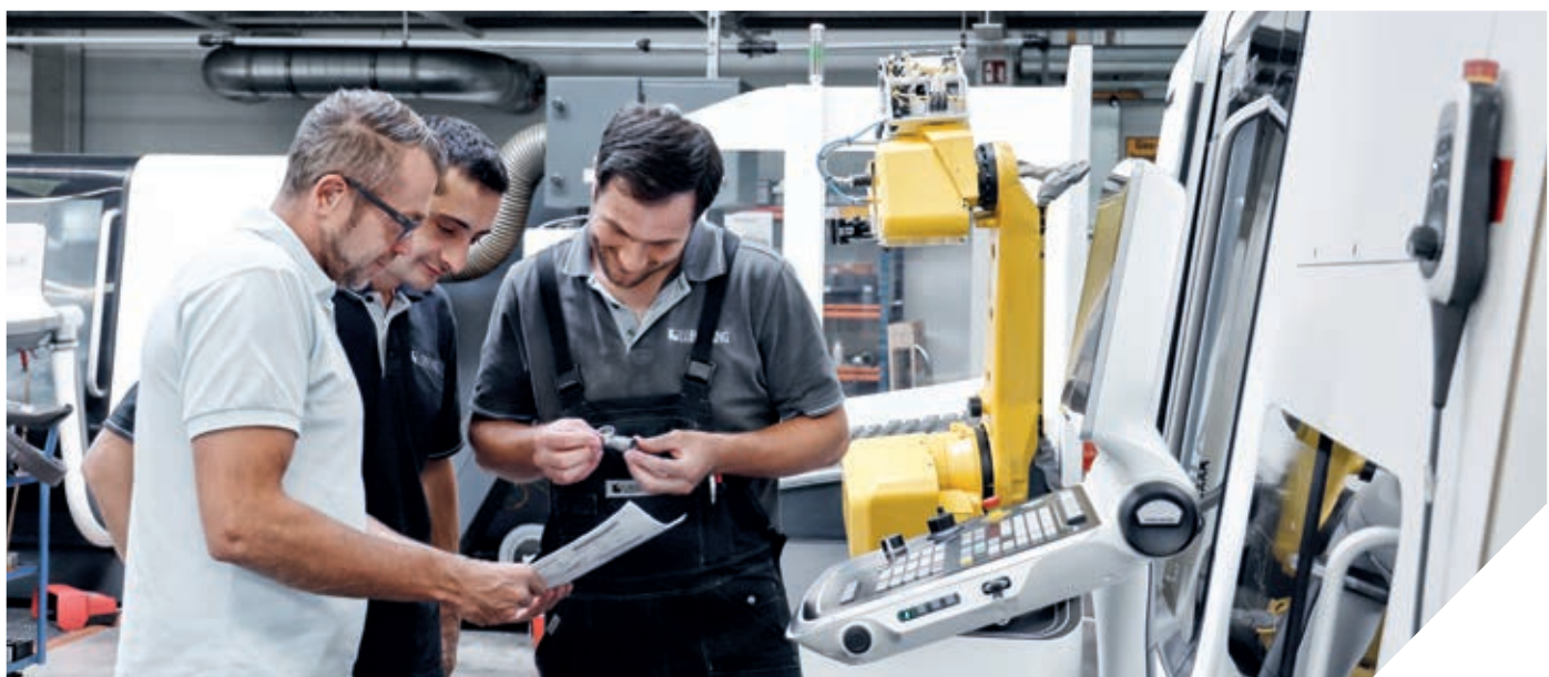
LÜBBERING supports its skilled staff on the CTC turn & mill centers with a Robo2Go from DMG MORI.
