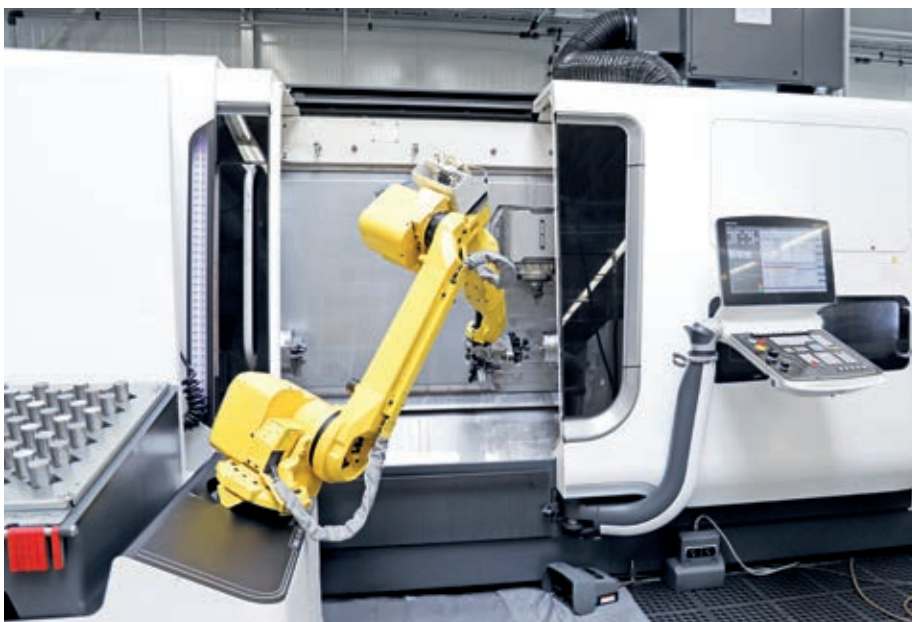
Unloading of the finished workpiece from the counter-spindle by the Robo2Go.
