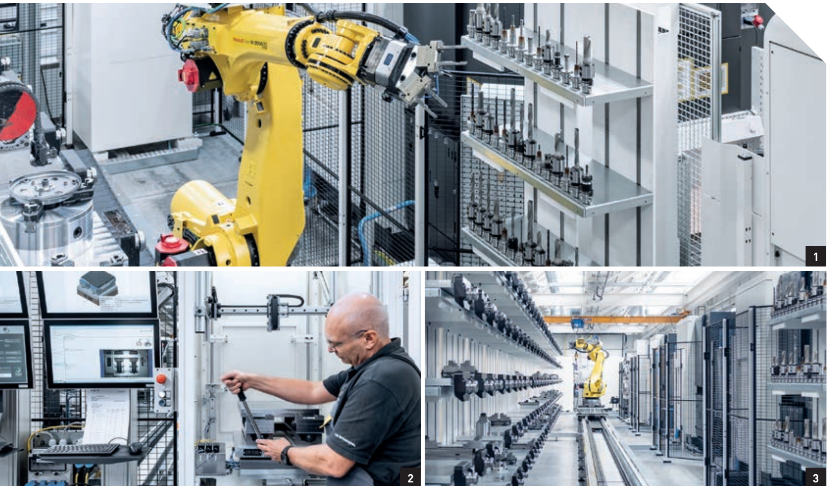
1. In addition to the 120 tool stations per machine, the automation also includes 105 stations for special tools. 2. The set-up stations are equipped with a camera system developed by Schaeffler, which enables the operator to set a zero point on the PC. 3. The 98-foot-long system includes five DMU 80 eVo linear machines, a tool presetter including a set-up station for tools, two set-up stations for workpieces and an off-load station.
