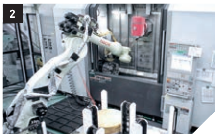
1. Example of a workpiece with a blank weight between 88 lbs. and 110 lbs. 2. Automatic robotic loading of the NT 4300 DCG
