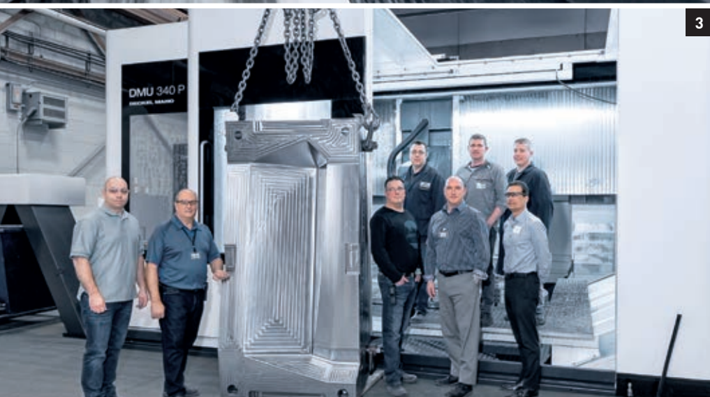
1. Sophisticated 5-axis machining on the DMC 85 monoBLOCK 2. With its three-pallet system, the DMC 85 monoBLOCK allows up to 20 hours of unattended operation 3. The DMU 340 P machines large workpieces to an accuracy of \pm 0.002 in.
